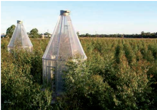
Whole tree growth chambers are used to study tree responses to CO 2 enrichment in the Hawkesbury Forest Experiment
